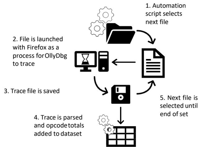
Fig. 2. Tracing process
