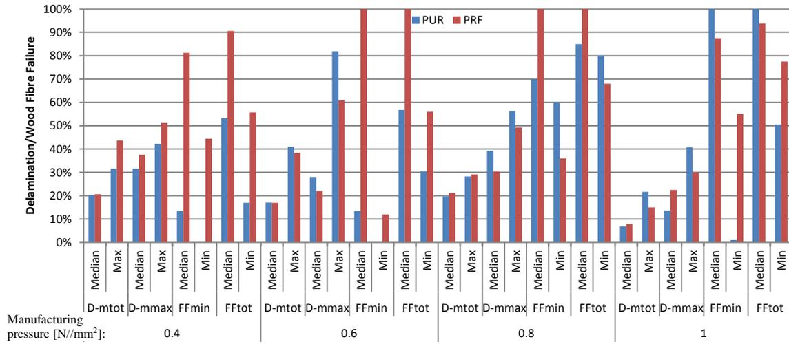
Figure 4 Delamination tests results<sup>‡</sup>
