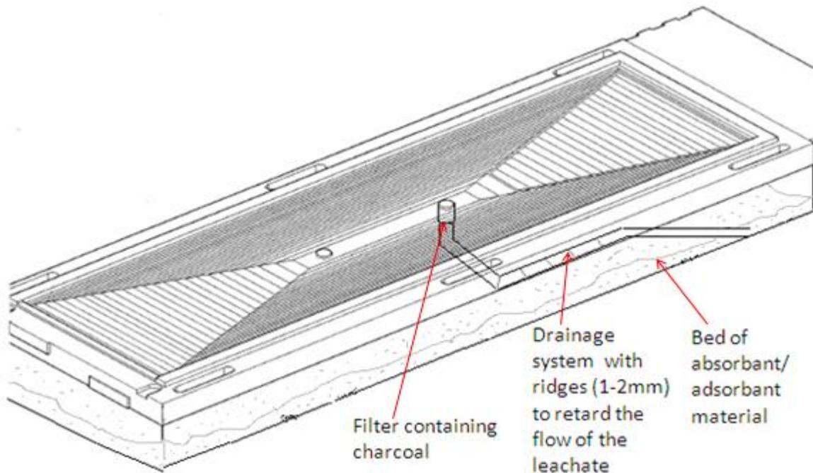
Figure 2-Initial concept of a proposed drainage system
