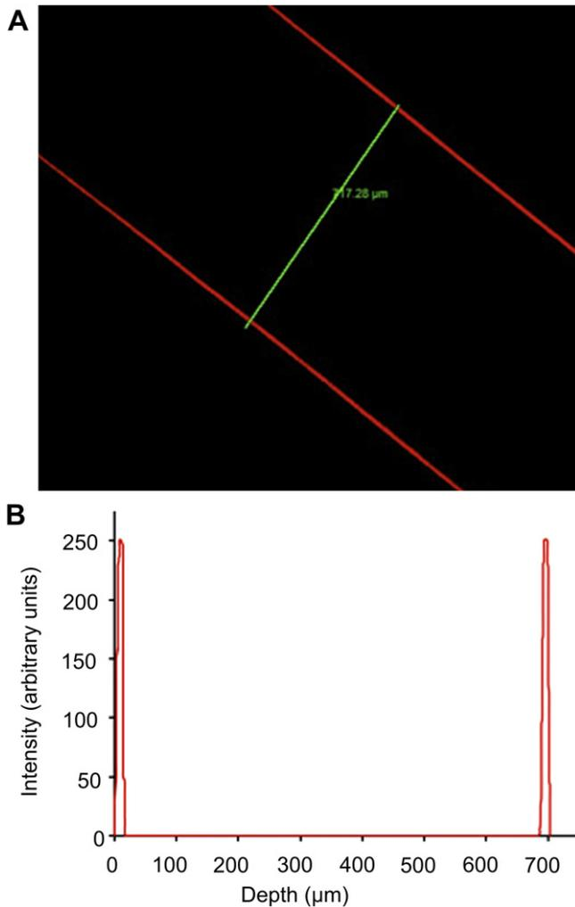
**Fig. 1.** A) Confocal scanning microscopy image of a TMPyP-impregnated 10MAA polymer. Line is drawn perpendicular to edges of polymer and corresponds with representative profile. B) Cross-sectional profile of the fluorescence of a TMPyP-incorporated 10MAA film measured by confocal laser fluorescence microscopy.
