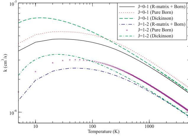
**Figure 2.** Electron-impact rotational excitation rates for the CS molecule for  $\Delta J = 1$  transitions starting from the  $J = 0$  and 1 levels. The results of a pure dipole Born calculation and the formula of Dickinson et al. (1977) are given for comparison.
